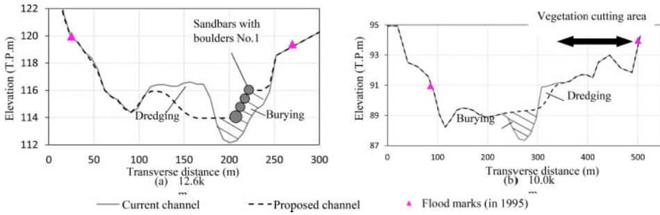
Figure 10. Cross-sections of the current channel and the proposed channel.
