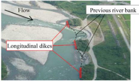
Figure 7. Bank erosion around the longitudinal dikes after 2005 flood (10.0 km point).
