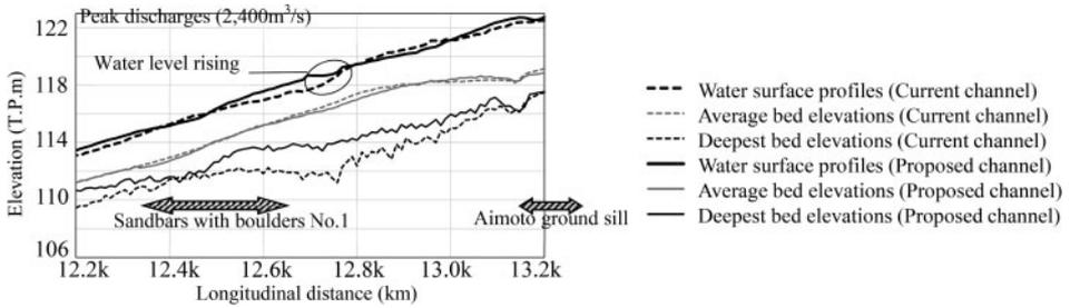
Figure 17. Calculated water surface and river bed profiles in the peak discharge in the current channel and proposed channel.
