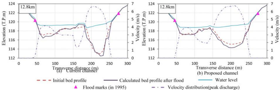
Figure 18. Calculated cross sectional bed profiles before and after the flood, velocity distributions and water level in the peak discharge.
